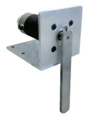
FIGURE 9: Experimental one-degree-of-freedom arm (pendulum) subject to gravitational force.
