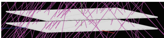
FIGURE 4: The schematically view of the muons interacting with the new detection system, observed with GEANT 4.94 code (magenta lines represent muons). We can see that not all muons that cross the first scintillator layer will pass through the second one.
