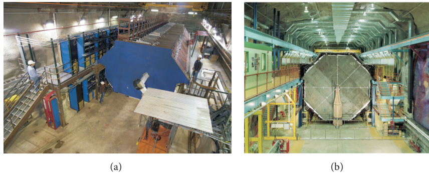
FIGURE 3: The MINOS detectors. (a) the near detector at Fermilab; (b) the far detector at the Soudan Underground Laboratory.
