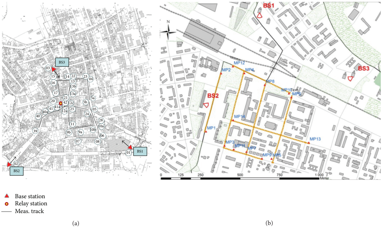
FIGURE 5: BS locations and measurement tracks in Ilmenau and Dresden.
