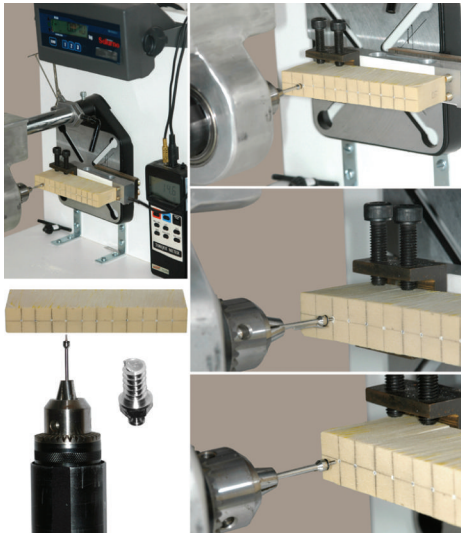
FIGURE 1: The equipment used for bone screw insertion in high-density artificial bone ( 0.80 \text{ g/cm}^3 ) and fracture.
