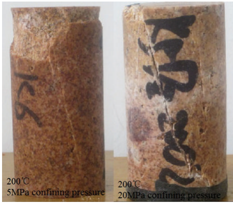
FIGURE 14: Ordinary damage states under triaxial stress.
