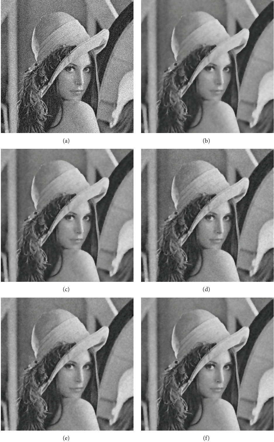
FIGURE 4: Comparison of different methods on “Lena” image. (a) The noisy image, \hat{\sigma} = 25 , (b) PM diffusion, (c) KAD method, (d) TDE, (e) ITDE, and (f) the proposed KTDE.
