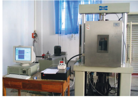
FIGURE 1: W3Z-200-type low-temperature triaxial test system for frozen soil.
