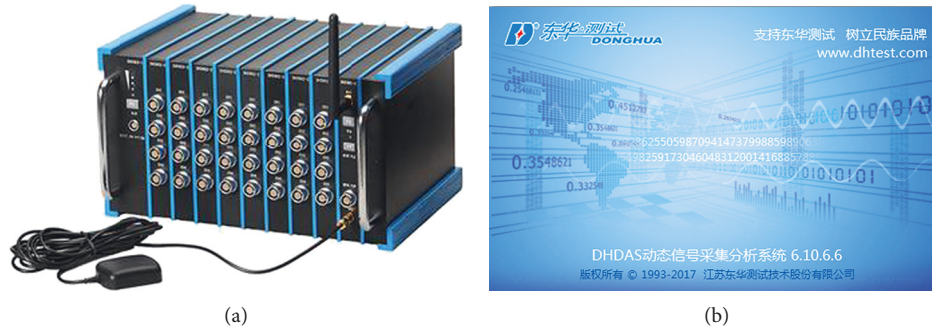
FIGURE 2: DHDAS dynamic signal acquisition and analysis system. (a) Data acquisition instrument. (b) Data analysis system.
