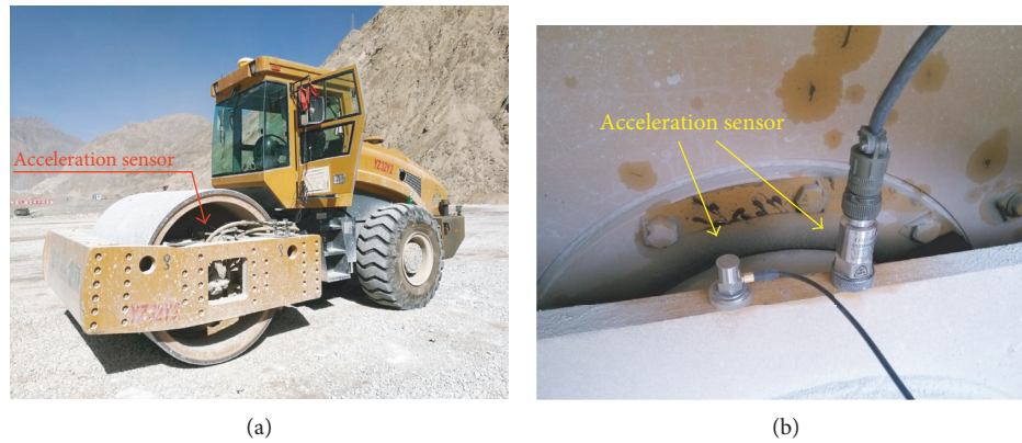
FIGURE 3: The vibratory roller and setting of sensors. (a) Vibratory roller. (b) Setting of sensors.
