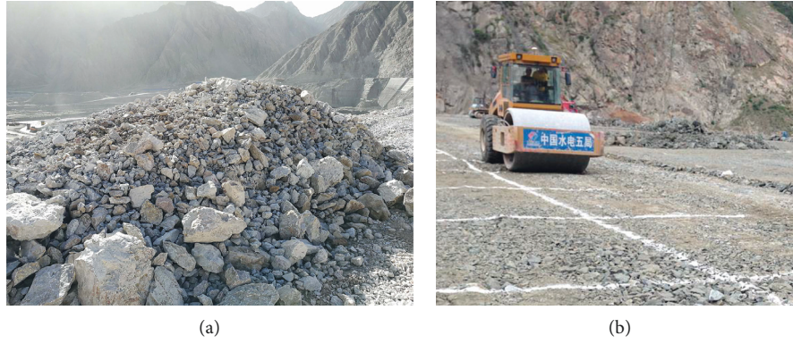
FIGURE 5: Field experiment on the main rockfill. (a) Main rockfill. (b) Field experiment.
