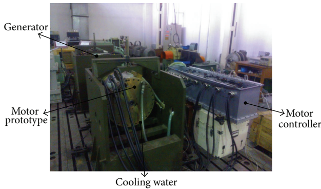
FIGURE 11: Test bench for the temperature measure.
