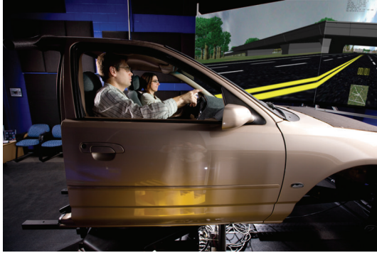
FIGURE 3: Moog 2000E motion platform and passenger cabin.
