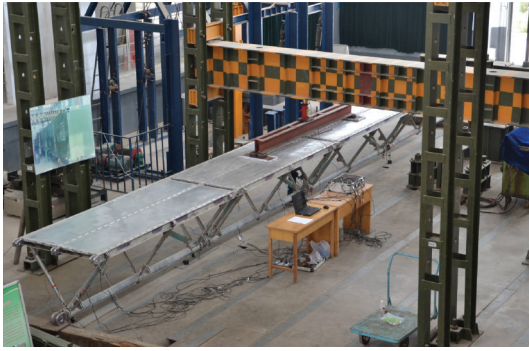
FIGURE 3: Single-span simply supported triangular truss and its on-axis four-point bending loading test setup.
