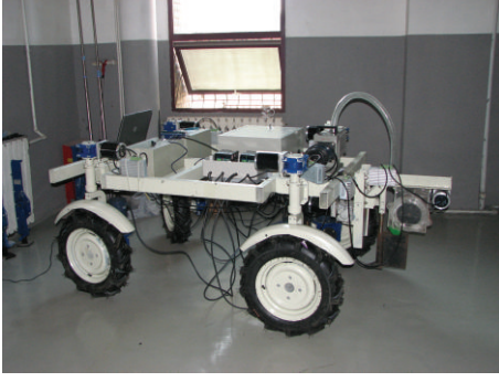
FIGURE 1: Wheat precision seeding robot.
