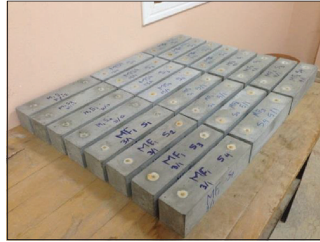
FIGURE 6: Free shrinkage test: (a) free shrinkage test setup and (b) test specimens.
