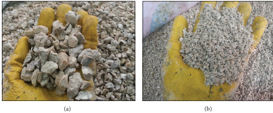
FIGURE 1: RAs: (a) RCAs and (b) RFAs as SSD condition.
