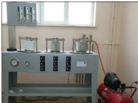
FIGURE 5: Water permeability test setup.
