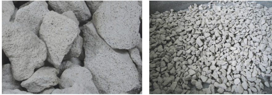
FIGURE 2: Crushed-AAC scraps into AAC aggregates.
