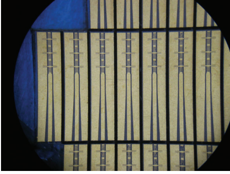
FIGURE 2: Processed ferrite substrate supporting antenna structures ready to be used in the return loss and resonant frequency measurements.
