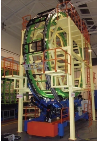
FIGURE 5: The circumferential drilling machine.
