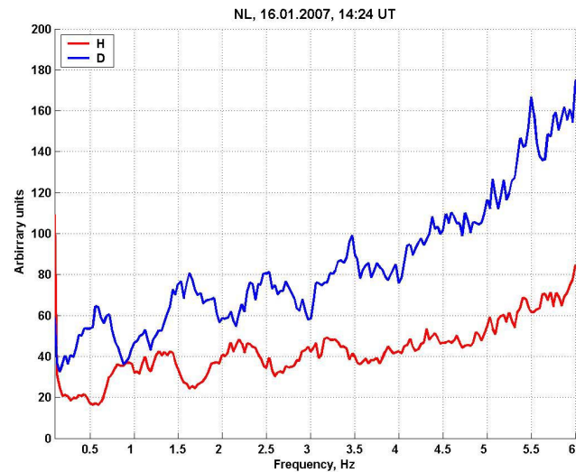
Fig. 4. A power spectrum of the H- and D-component as observed at NL at the given date and time. Averages over successive, non-redundant, 512 point FFTs were used to get an integration over \sim 10 min. The general increase of the power spectral density over frequency reflects the increase of sensitivity of the search coil magnetometer (raw data).
