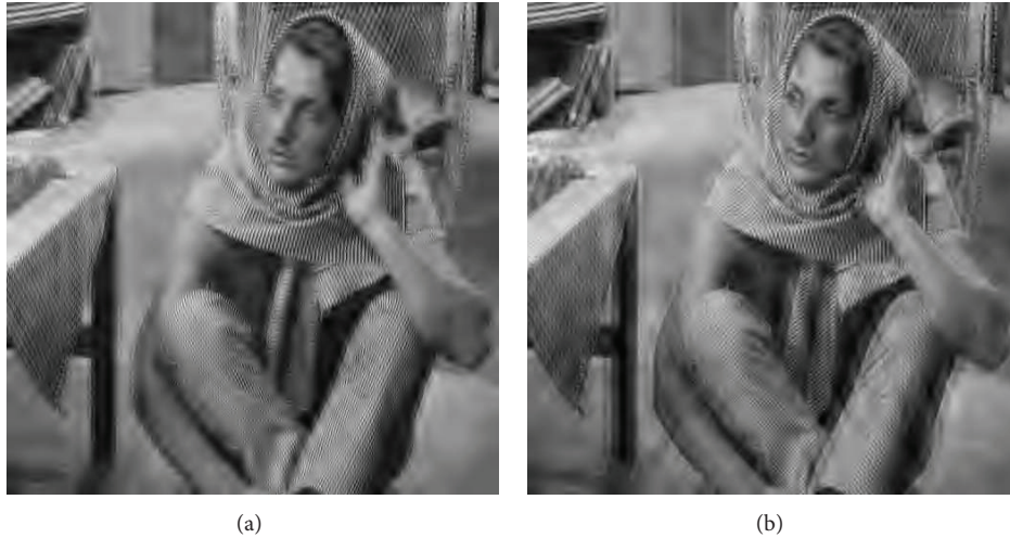
FIGURE 13: Two channel reconstruction for Barbara ( 512 \times 512 \times 8 ) with packet loss ratio of 40% at R_t = 0.34 bpp: (a) MDSQ PSNR = 22.69 dB and (b) the proposed method PSNR = 23.17 dB.
