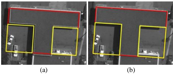
Figure 6. Initial MBRs (a) and adjusted MBRs (b) of the first building projected onto the image
