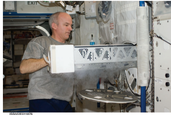
Figure 5 Expedition 13 crewmember Jeff Williams, Expedition 13 NASA space station science officer and flight engineer, inserts a sample, such as the EC samples, in the -80°C laboratory freezer for ISS (MELFI) in the Destiny laboratory of the ISS.
