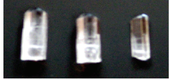
FIGURE 13: Deuterated L-threonine single crystals grown from seed rotation technique.
