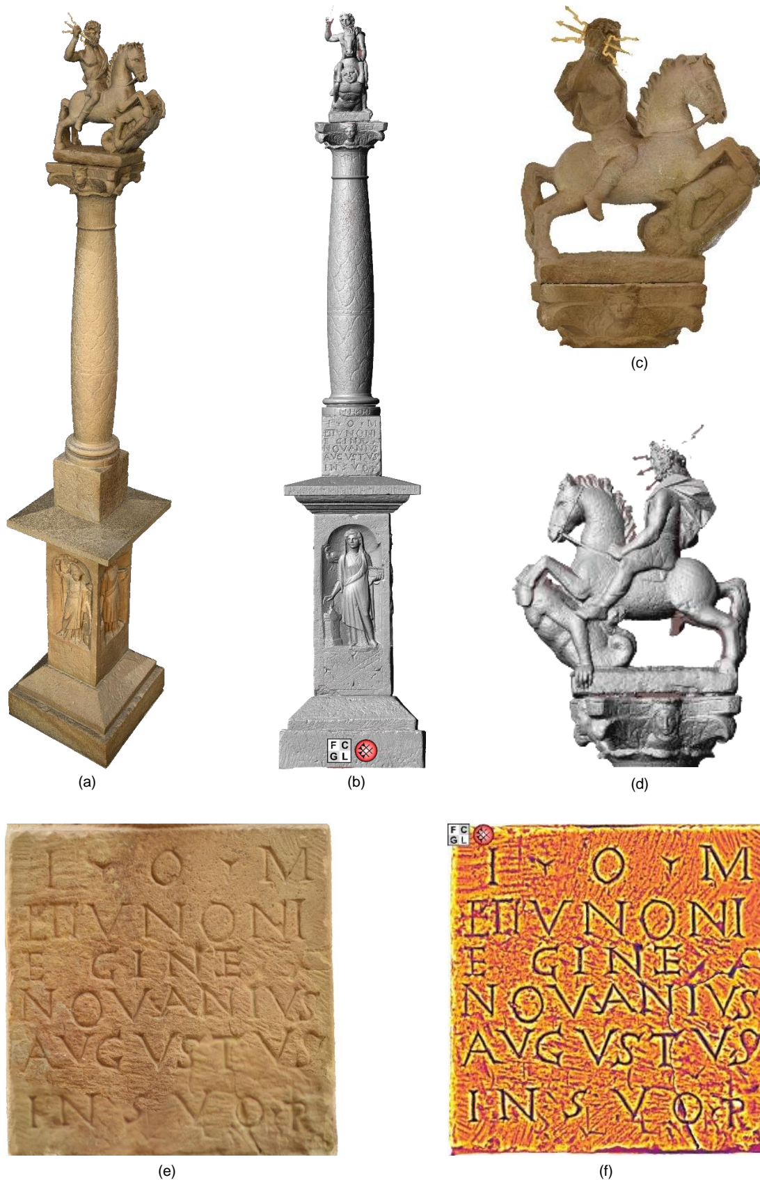
Figure 1: 3D reconstructions of the Jupiter Column: a) 3D view of the Jupiter Column ; photogrammetric reconstruction based on approximately 700 photos with a resolution of 36 megapixels/image. Photo: IPF/KIT; b) Front elevation of the Jupiter Column ; structure light-based reconstruction with the SmartSCAN-3D-HE. Photo: FCGL/Heidelberg University; c) Right side of the main motive (a riding, Titan defeating Jupiter); photogrammetric reconstruction based on approximately 700 photos with a resolution of 36 megapixels/image. Photo: IPF/KIT; d) Left side of the riding, Titan defeating Jupiter; structure light-based reconstruction. Photo: FCGL/Heidelberg University; e) Detail of the photogrammetric reconstructed inscription. Photo: IPF/KIT; f) Detail of the inscription, reconstructed with structured light. Fictive colors. Photo: FCGL/Heidelberg University.
