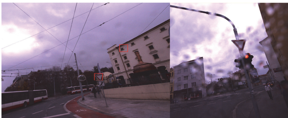
5: A false positive region on the left picture (top right) can be eliminated due to its position. On the right image is shown a distortion from raindrops
