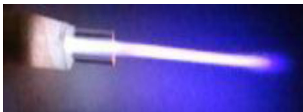
Fig. 1 Image of the cold helium plasma jet at atmospheric pressure utilized for surface activation of glazes
