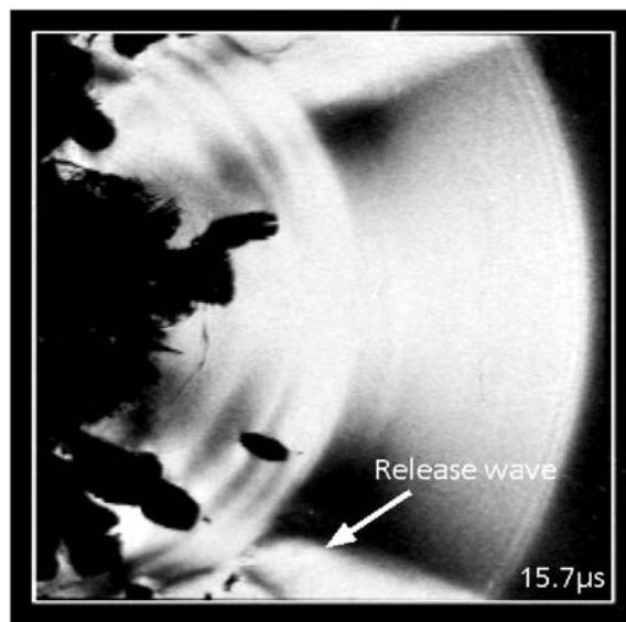
Fig. 8 A comparison of the longitudinal stress wave fronts obtained (a) computationally and (b) experimentally (in Ref 1, 2) for the case of a spherical impactor with an initial velocity of 440 m/s and a post-impact time of 15.7 \mu s
