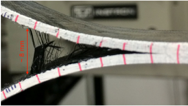
Figure 11 Side-view photograph of DCB test specimen of the CFRP composite with a matrix modified with 4 wt% silica nanoparticles taken during the interlaminar fracture test. The fibre bridging and fibre-bundle bridging toughening mechanisms are clearly evident.
