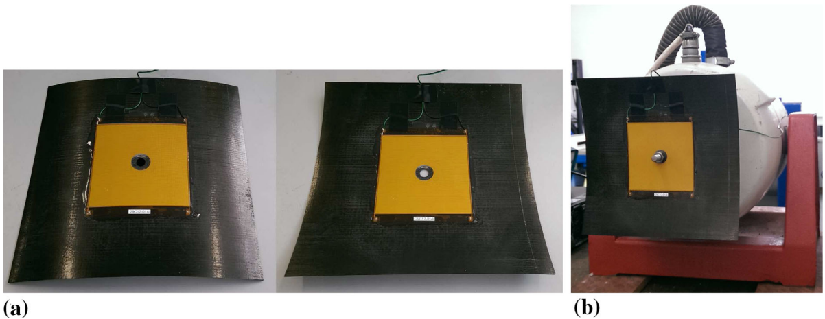
Fig. 1 a The laminate used for these tests measures 190 mm × 190 mm × 0.5 mm, has a [0/90]_T layup and has a single piezoelectric layer Micro-Fibre-Composite (MFC) attached to the top surface of dimensions 85 mm × 85 mm × 0.3 mm, and b experimental setup showing mechanical shaker attachment
