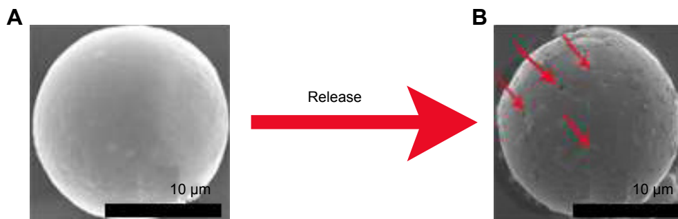
Figure 6 In vitro dialysis release study of BH from formulations: (a) BH solution, (b) conventional BH microsphere, and (c) BMEM. The cumulative drug release (%) is plotted against time (h). Values are presented as the mean \pm SD (n=5). SEM micrographs of BMEM: (A) microsphere before release process and (B) microsphere after release process.
