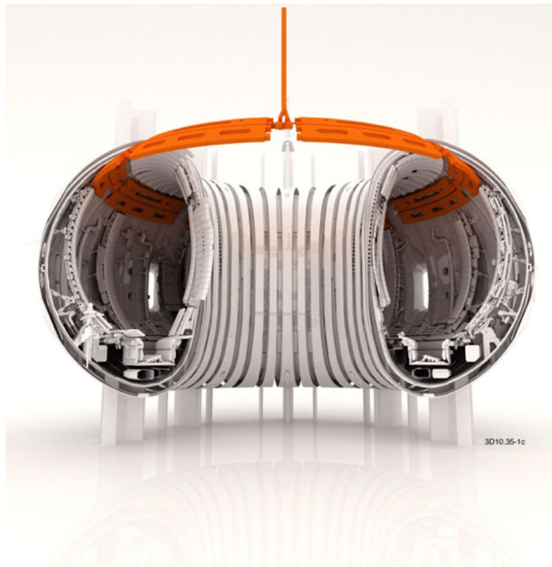
Fig. 2 Artist's impression of Resonant Magnetic Perturbation coils mounted in JET
