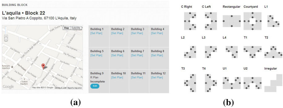
Fig. 15 Extract from the web-interface of LOG-IDEAH. a The localisation of the inspected AA block, definition of the number of AAs which belong to the AA block under investigation. b Plan geometry associable to the inspected AAs
