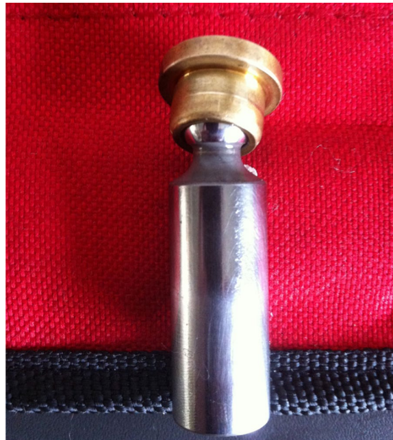
Fig. 6 The failure of loose slipper
