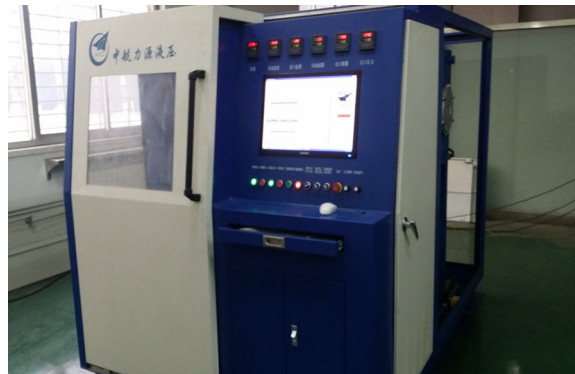
Fig. 2 Test-bed for hydraulic pump degradation experiment
