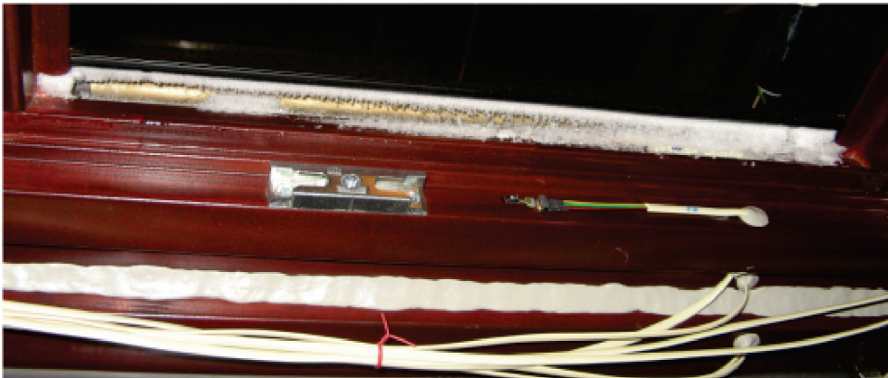
Fig. 2. Demonstration of ice coating and condensation in gap between casement and window frame at exfiltration and 200 Pa pressure difference (lower part).
