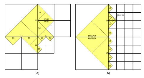
Figure 21: Tile resolution assignment in the *Seamless Patches* algorithm. a) In this case the number of *levels of detail* of the *tiles* is 2 (e.g. 16 and 32 vertices) and the branching factor
