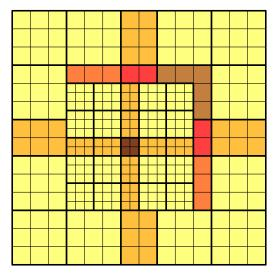
Figure 16: Tiling of a geometrical *clipmap*. Tiles depicted with same color share their index and vertex buffers. Size (4x4 vertices) of the most frequently used type (yellow tiles) is chosen to optimally utilize vertex caching.
