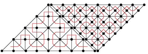
Figure 6: Example of a Sierpinski space filling curve on two consecutive levels of detail of a 4-8 triangle mesh.
