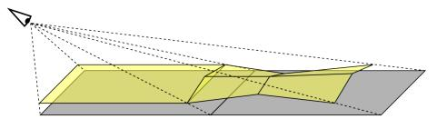
Figure 9: Visual masking of gaps between neighboring tiles of a different *level of detail* using textured and view-projected planes.
