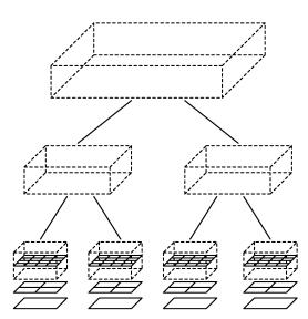
Figure 7: One dimensional scheme of a tile quad-tree in the *Geometrical Mip-Mapping* algorithm. While non-leaf nodes contain only bounding boxes, leaf nodes contain bounding boxes, full resolution geometries as well as other subsampled geometry levels.
