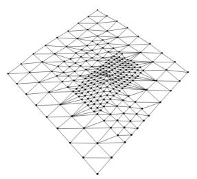
Figure 8: Filling of gaps between neighboring tiles of a different *level of detail* using triangle fans. Topology of lower resolution tiles is adapted to higher resolution tile borders.
