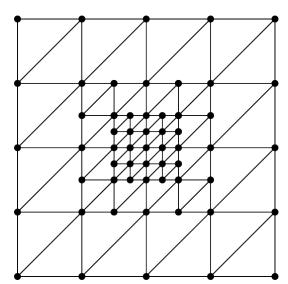
Figure 13: Nested square *clipmap* tiles of the *Geometrical Clipmaps* algorithm. Practical tile resolution is between 255 and 2047 vertices and not 5 as depicted.
