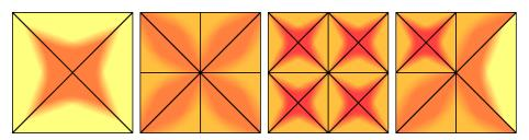
Figure 18: Three consecutive levels of a binary tree of tiles of a BDAM algorithm and a resulting triangulation made of them.
