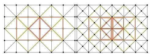
Figure 5: Demonstration of two *levels of detail* of a 4-8 triangle mesh in a ROAM 2.0 algorithm. A *diamond* – four triangles sharing an apex vertex – (depicted in red color) has four children diamonds in the higher resolution level (the light brown ones), two parents (in orange) in a lower resolution level and six siblings (neighbors) (the yellow diamonds). The colored vertices are those the appropriate diamonds (the colored squares on the figure) are assigned to.
