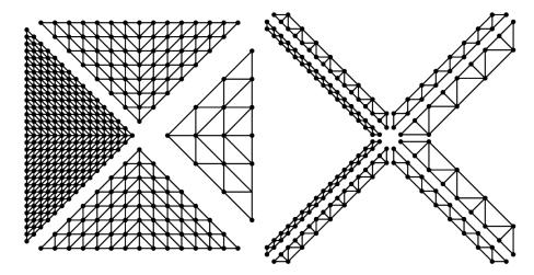
Figure 20: Triangular tiles of a seamless patch (left) and adequate stitching strips (right).
