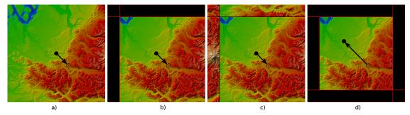
Figure 15: Toroidal updates of *clipmap* buffers. a) Initial state of the buffer before an user moves from the black point to the empty point. b) After the user moves, the black parts of the buffer has to be reloaded. c) They are filled with three blocks toroidaly. Addressing is then done using modulo function. d) Worst case scenario. When the user moves backwards over a buffer's edge, five blocks has to be updated. Source of data: USGS. [20].
