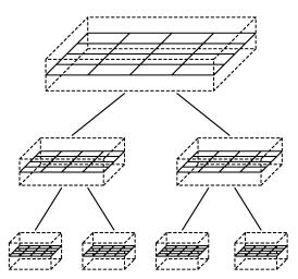
Figure 10: One dimensional schema of a tile quad-tree in a *Chunked LoD* algorithm. Each node contains a bounding box of the tile and its geometry. Object-space error of the geometry is decreasing and size of the tiles is shrinking exponentially from the root to the leafs.
