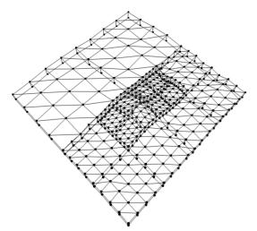
Figure 11: Example of tiling of a *Chunked LoD* algorithm. Covering of gaps between neighboring tiles of a different *level of detail* is done by rendering vertical skirts around each tile's border.
