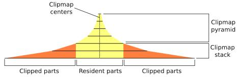
Figure 12: Clipmaps construction from mipmaps by cropping to *clipmap size*.
