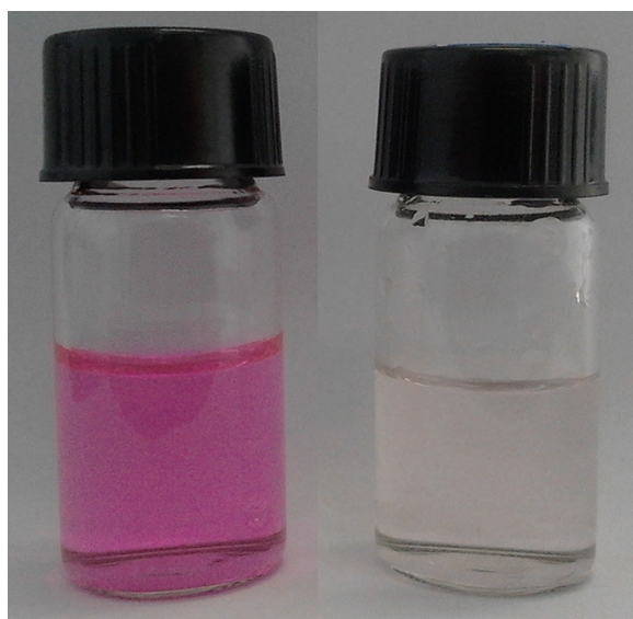
Figure 6 Rh.B solution (0.01 mg/mL, left) before and after separation of G/M-CdS adsorbent after photodegradation (right).
