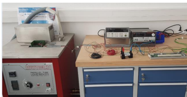
Fig. 1. Experimental set up used to obtain laboratory calibration curves under laboratory conditions.
