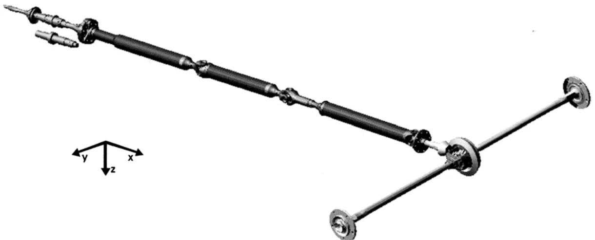
Fig. 1 The multi-body model of the driveline mechanical system
