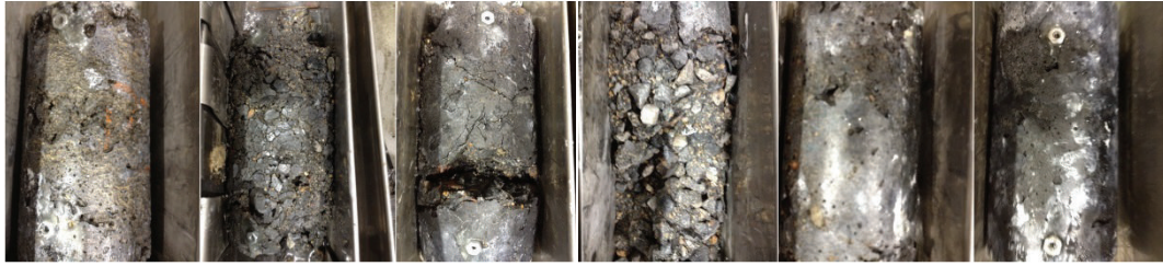
FIGURE 11: CNT concrete after 300 cycles of freezing and thawing (left to right: 0.0 wt% CNT, 0.5 wt% CNT, 1.0 wt% CNT, methylcellulose + 1.2 wt% CNT, silane + 1.2 wt% CNT, and sodium polyacrylate + 1.2 wt% CNT).
