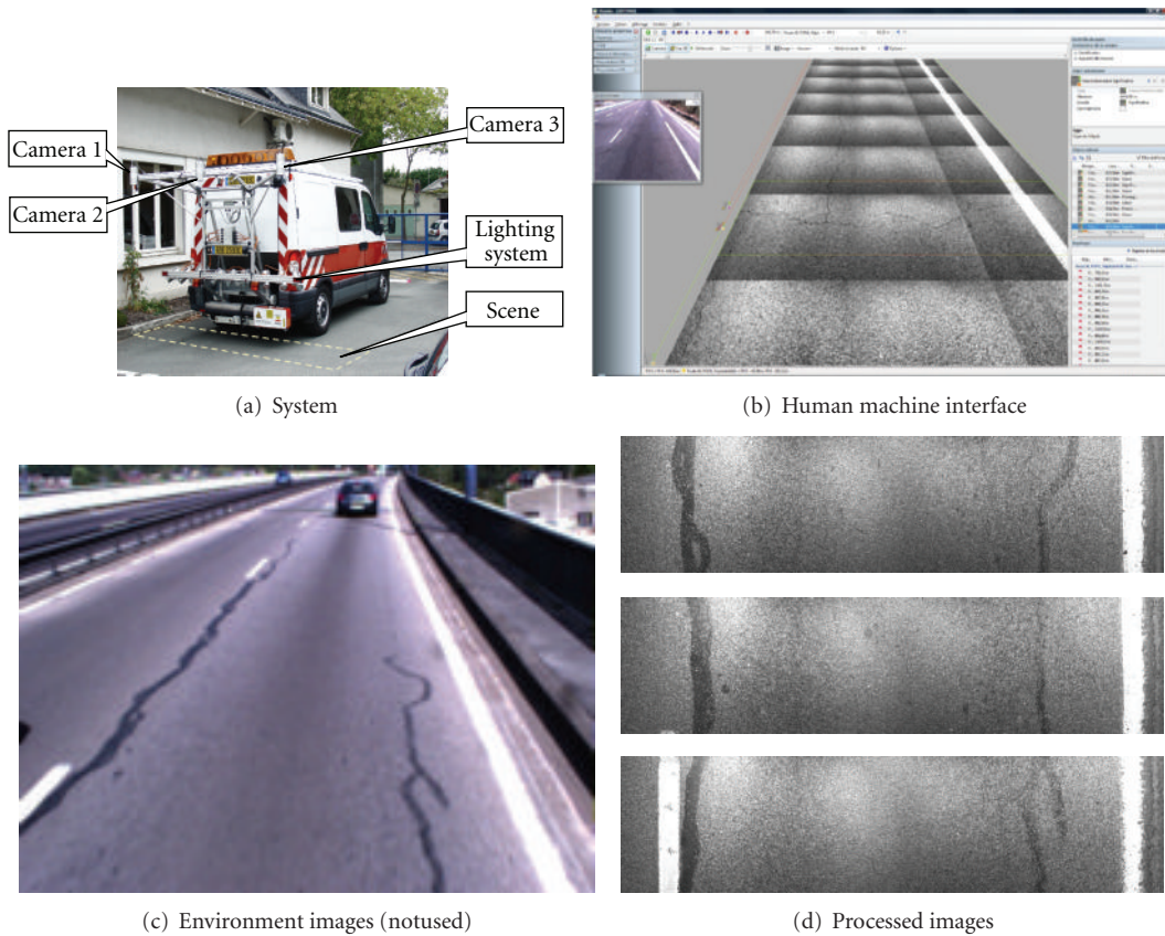
FIGURE 5: The acquisition system used for the evaluation. In (a), the acquisition system is illustrated whereas in (b) it shows the user interface. In (c, d), an example of the final images is given. In (d), we can see the road that is visible in (c). The processing is done 1 meter by 1 meter, that is, independently on each image presented in (d). The surface contains two reparations of vertical cracks. In some cases, the 3 sensors do not have the same settings, and the global illuminations are different, so it can generate some “false cracks”. This aspect has been easily taken into account in a preprocessing step by eliminating the junction area in the region of interest.
