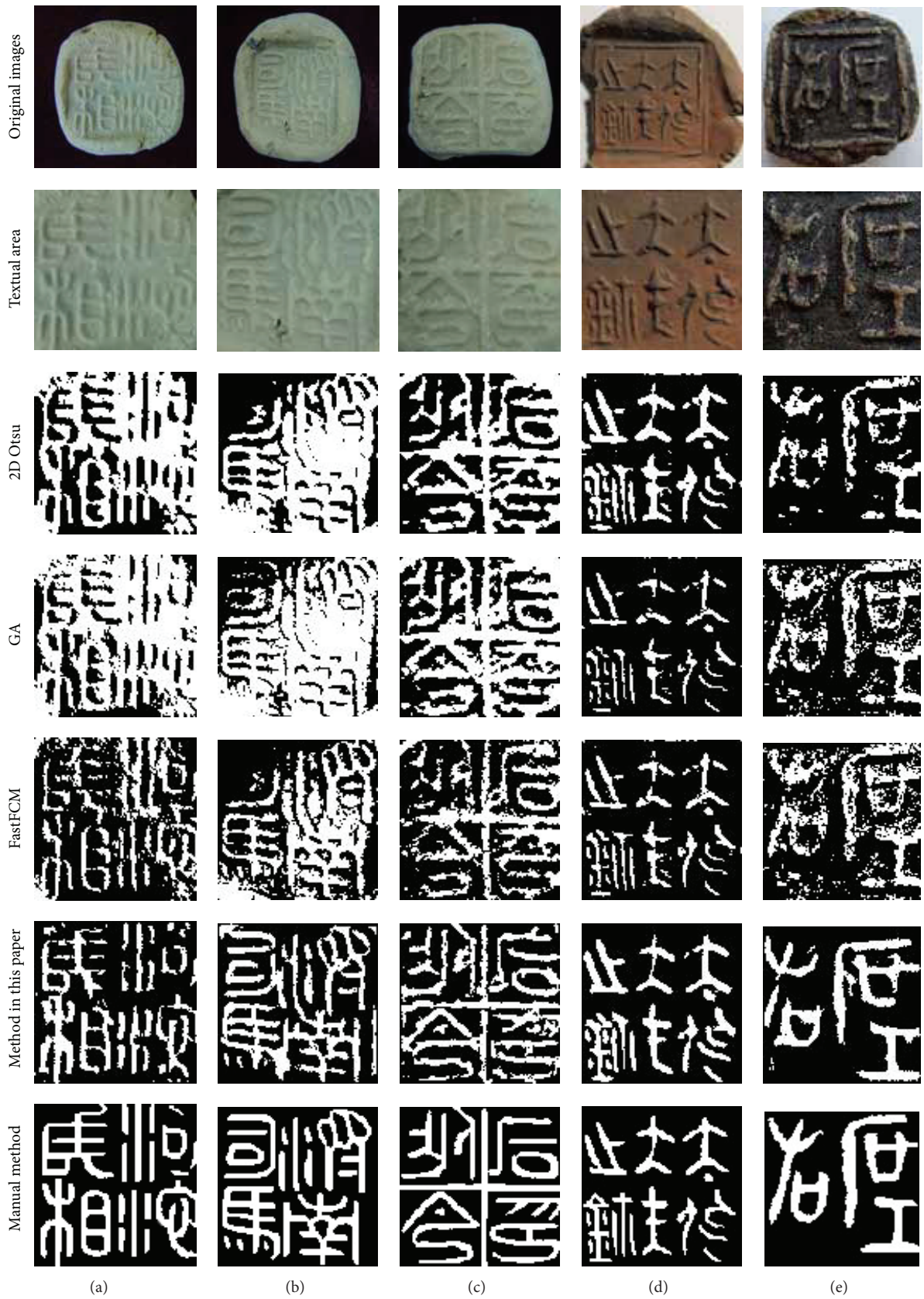
FIGURE 7: The segmentation results using different methods including 2D Otsu, GA, FastFCM, and the proposed method.
