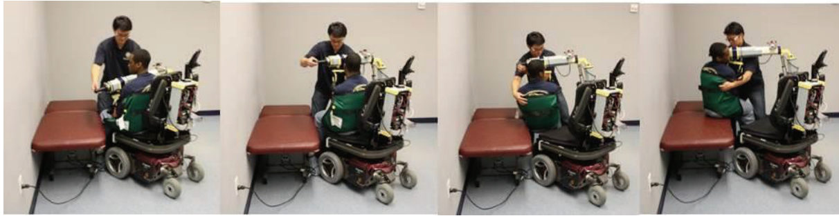
FIGURE 5: A sequence of photographs of the RATD being used to transfer a person from an electric powered wheelchair to a mat table, by a caregiver.
