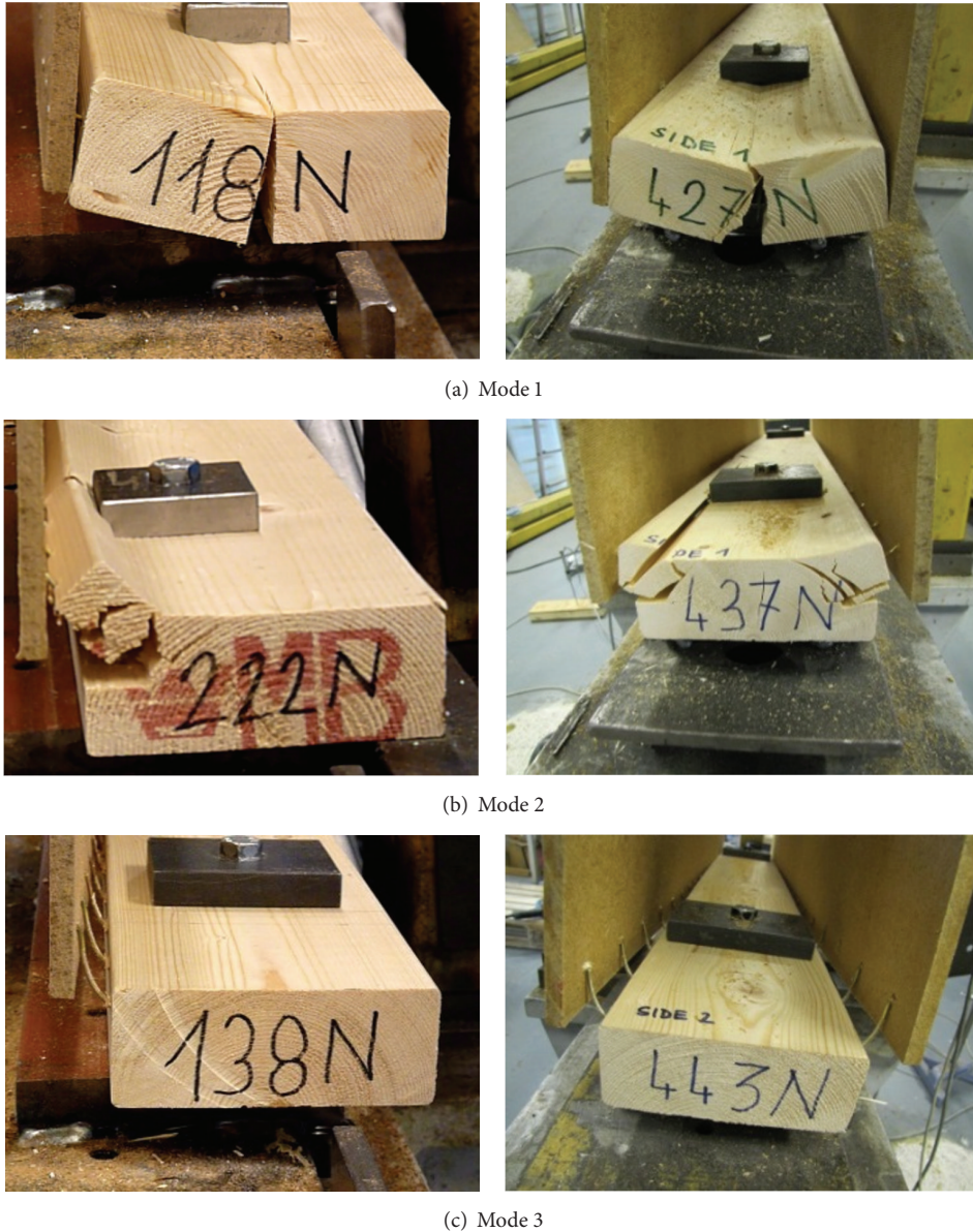
FIGURE 2: (a) Splitting failure along the bottom side of the rail; (b) splitting failure along the edge side of the rail; and (c) yielding and withdrawal of the nails in the sheathing-to-framing joints.
