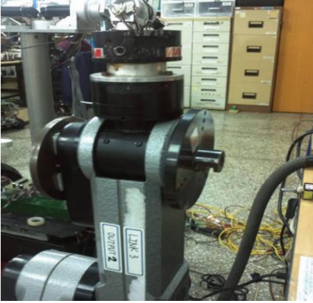
FIGURE 6: Photograph of the link2 with attached mass.
