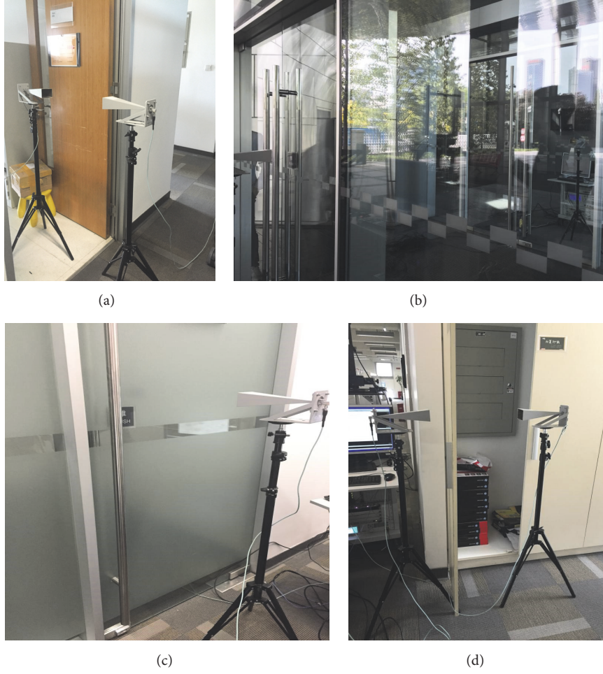
FIGURE 4: Penetration loss measurements for a wooden door of the laboratory (a), a transparent glass door of the hall (b), a frosted glass door of a small office (c), and a wooden door of the cabinet (d).
