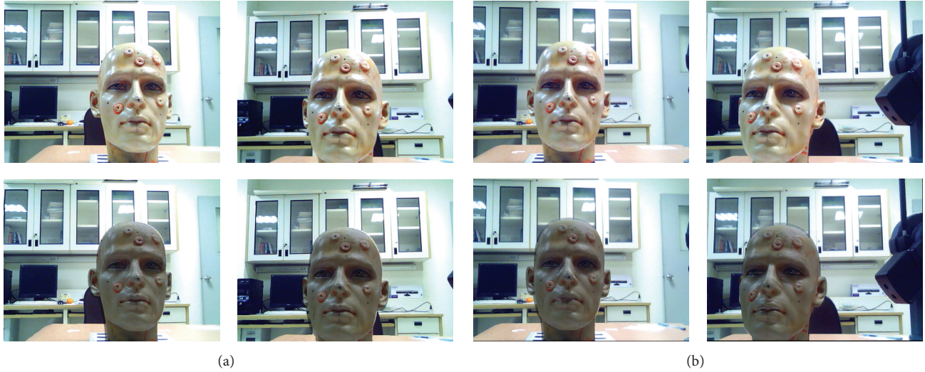
FIGURE 8: Augmented reality visualization results of the proposed medical AR system using the plastic phantom head as testing subject. (a) First row: original stereo images view, second row: AR visualization result. (b) AR visualization results in another view.
