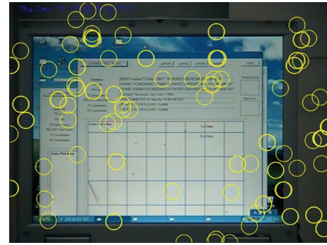
FIGURE 5: Menu image of the pilot application program, executed on a notebook PC under test (during gamma ray irradiation, about 15 min elapsed).
