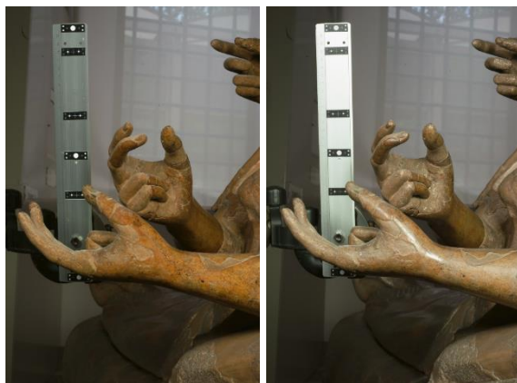
Figure 5. A test image of the hands and a scale bar acquired with (left) and without (right) cross polarization.
