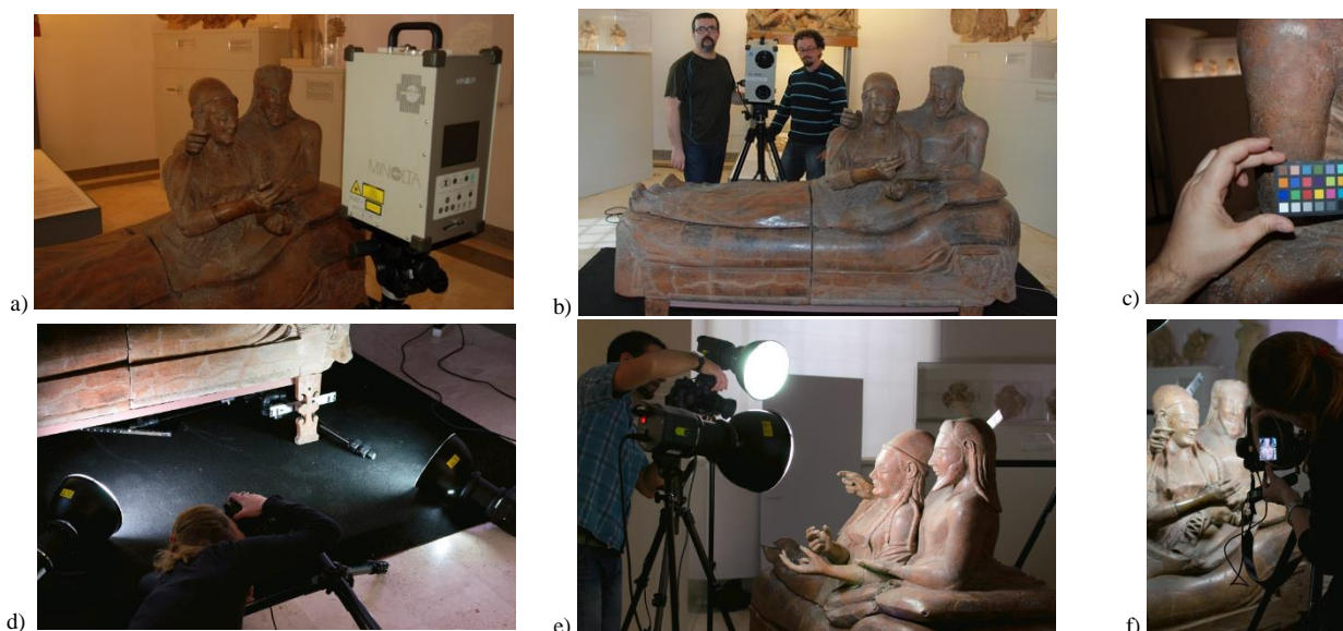
Figure 3. Data acquisition: the adopted triangulation-based laser scanner, a Konica-Minolta Vivid 910 (a, b); Gretag Macbeth colour checker (c); photogrammetric survey with artificial light and camera mounted on a tripod (d,e,f).
