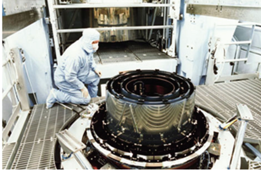
FIGURE 12: The Chandra telescope during integration of the four mirrors. The fourth mirror shell waits in the background.
