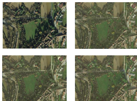
Figure 4: Original image and image after deshadowing approaches. In order: EAOP, ObP and Cholesky deshadowing methods
