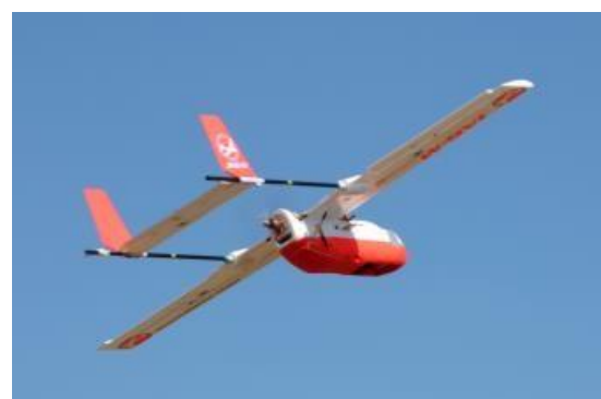
Figure 3. The JAG-M fixed-wing UAV.
